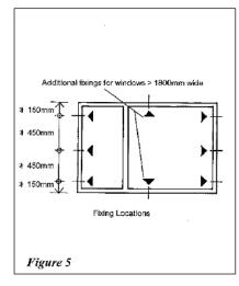
Special requirements may be necessary when fixing windows into preformed openings.
