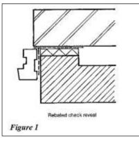
In exposed conditions consideration should be given to using a rebated check reveal (Figure 1)
